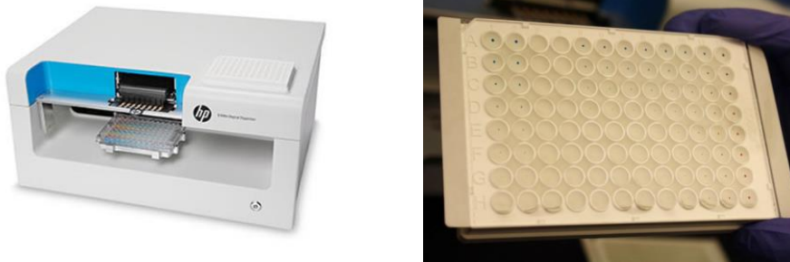
Figure 6. ExAST utilizes an HP D300e digital dispenser to prepare on-demand broth microdilution panels consisting of different antimicrobial combinations.
